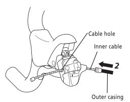
If the cable hook does not align with the shifting cable hole, press lever (B) again until it does, and then install the cable.
