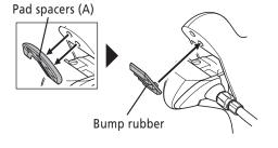
To increase the lever stroke Remove the pad spacer (A) and install the bump rubber.
