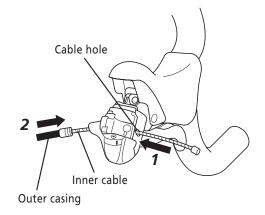
If the cable hook does not align with the shifting cable hole, press lever (B) again until it does, and then install the cable. **Confirm:** Make sure that the inner end is firmly set in the cable hook.
