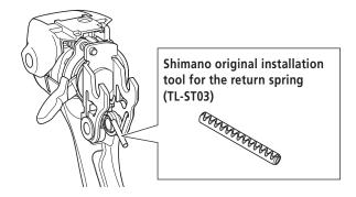
2. Align the stud holes, and then press-fit the lever axle in the position shown in the illustration.
