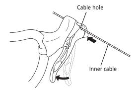
**4.** Run the inner cable through the outer casing.
