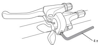
Tightening torque: 6 - 8 N·m {53 - 69 in. lbs.}
