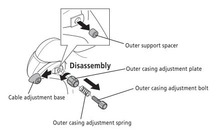
\* Insert a thin bar-shaped object to remove the outer support spacer.
