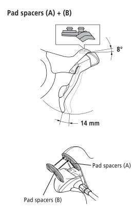
To decrease the lever stroke Insert pad spacer (B) as far as it will go and so that the protrusions fit into the holes in pad spacer (A).
