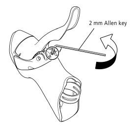
2. Insert an Allen key or similar tool into the lever axle hole, tap it gently with a plastic hammer to push out the lever axle, which disassembles it into the bracket body and the lever body.
