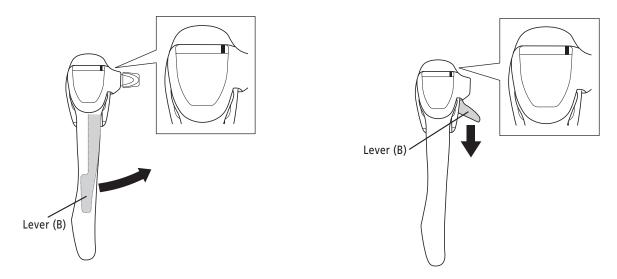
**3.** Depress the brake lever, and then pass the inner cable through the cable hole.
