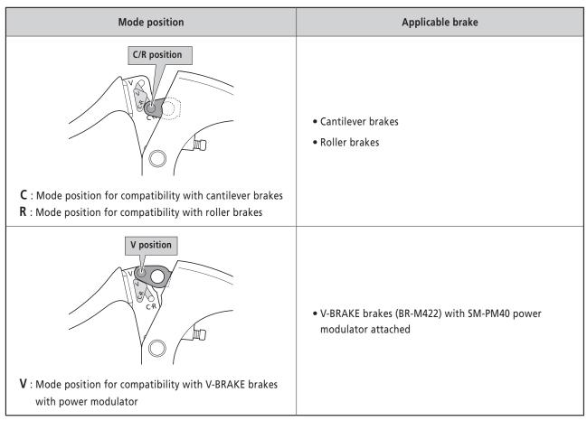
Use the brake levers with mode switching mechanism in the combinations given above.
